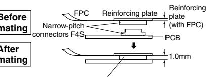
The simple lock mechanism ensures that the connector clicks into position when it is inserted for reliable single-action insertion on the PCB.
